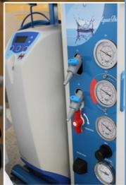
The water being supplied into the dialysis process needs to be of the highest purity. This Reverse Osmosis Water Purification System purifies the water through a process called reverse osmosis. In the dialysis process, the blood and water run alongside a semipermeable membrane which allows the toxins to transfer to the water and out of the body, leaving the blood clean. Thanks for making this purchase possible!
